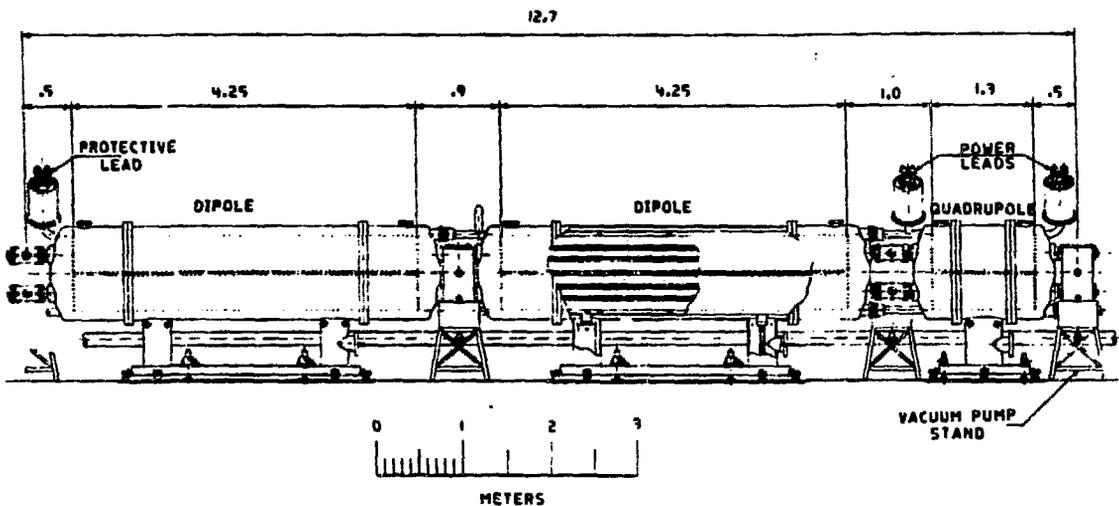
Fig. 2. Typical half cell
