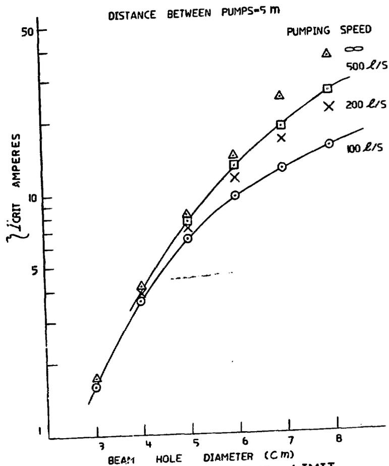
FIG. 4 CRITICAL CURRENT LIMIT
