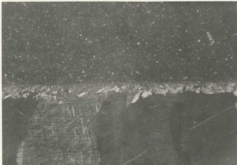
(b) Uranium-to-Niobium Interface.
