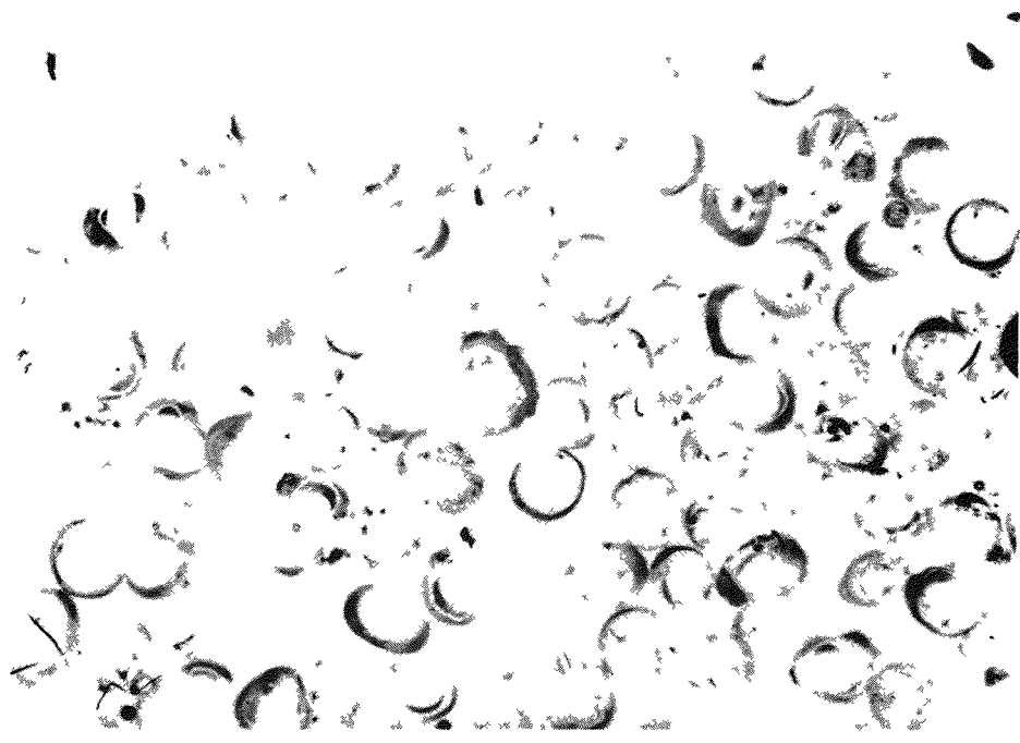
Fig. 7 - 0.0314 in. glass particles before test (Magnification 11.6:1).
