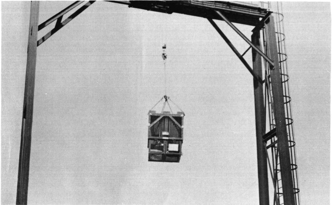
FIGURE F-1 - MHW-IHS-SC at a height of 30 ft prior to the drop test.
