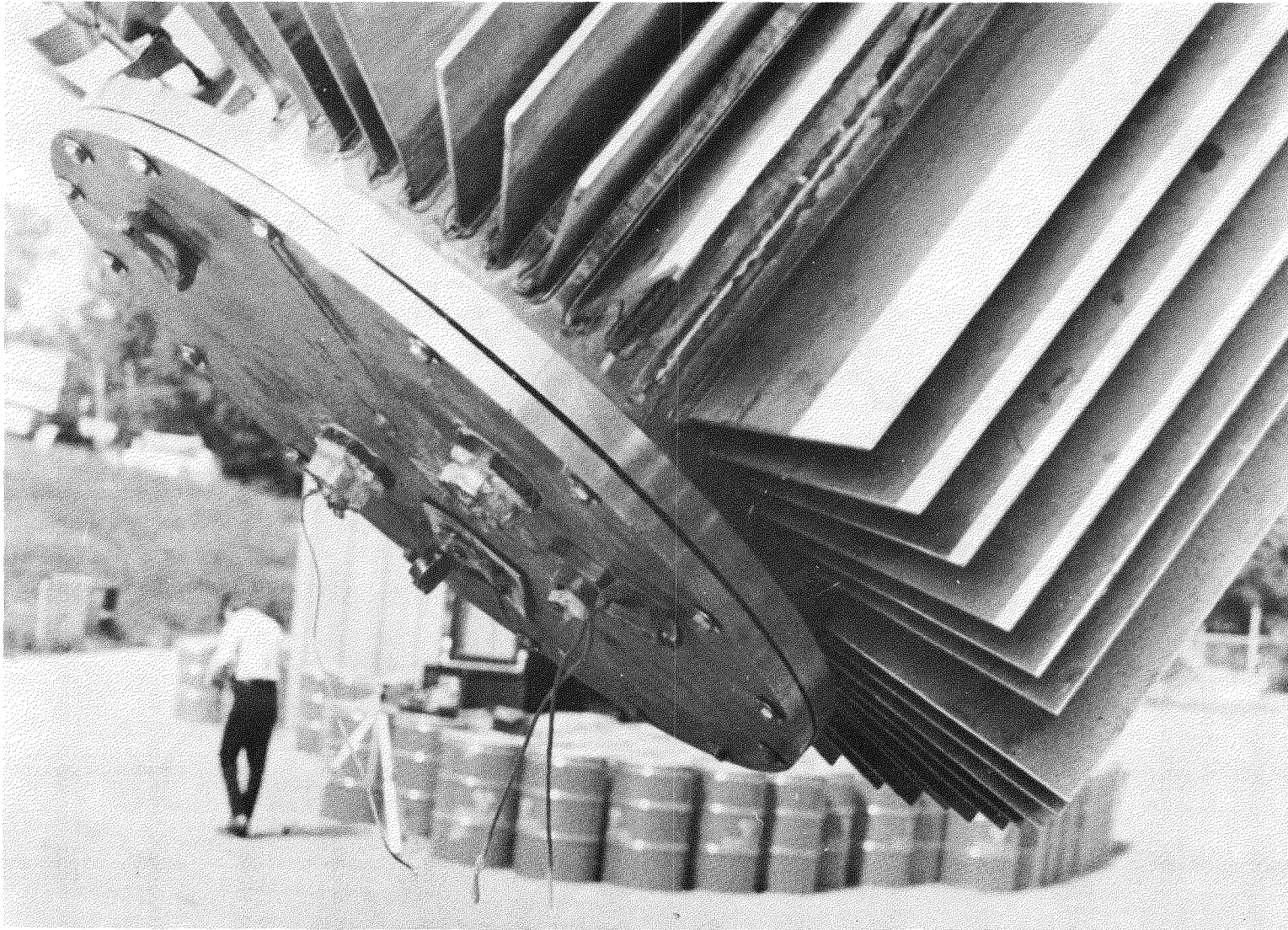
FIGURE F-4 - The cask cover seal was lost as a result of stretching the bolts. A gap can be seen between the cover and the mating flange.
