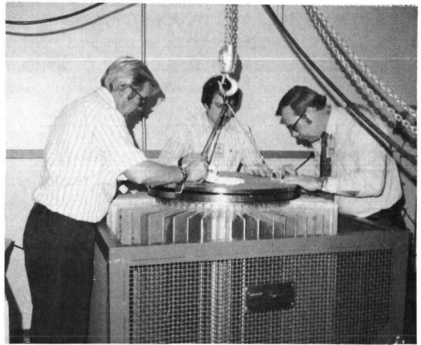
FIGURE i-7 - The finned cask cover is lowered in place using a hoist.
