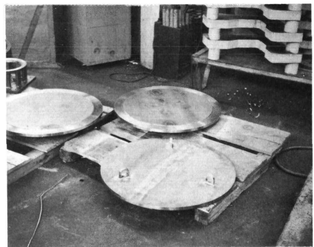
FIGURE i-13 - The cask covers are shown during fabrication.
