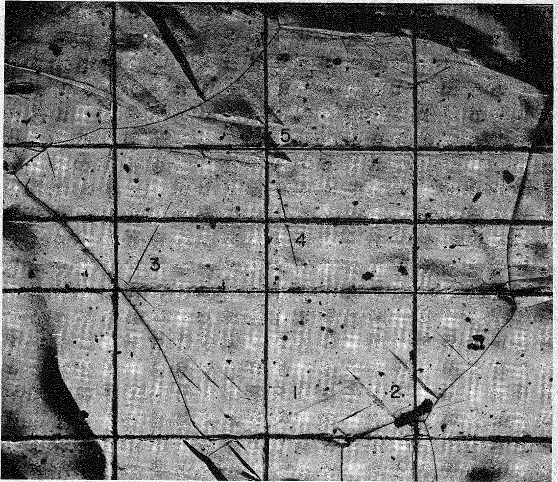
FIG. 10 FIVE OPERATIVE TWIN MECHANISMS IN GRAIN M3 OF SPECIMEN 4 AT 0.25 % \epsilon . (100X REDUCED BY 20%)
