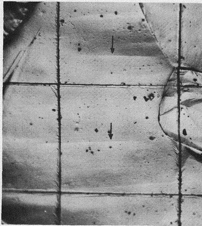
(a) SPECIMEN 4, GRAIN L6 AT 2.4% \epsilon (100X)
