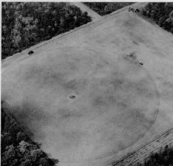
Figure 2. 200-curie cobalt-60 radiation field. The source is located at the center of the circles and the control house can be seen in the upper part of the picture. Close to the source are the pie-shaped sectors that hold potted plants which can be watered from the control house by remote control.
