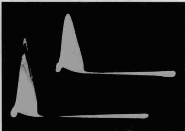
Figure 6. Photograph of scintillation counter pulse distribution for \text{Cu}^{66} as displayed on an oscilloscope screen. Photo-peaks and Compton distributions of the 1.04-Mev gamma ray of \text{Cu}^{66} and of the \text{Cu}^{64} annihilation radiation can be seen. The \text{Cs}^{137} pulse distribution is shown at the right, for comparison.
