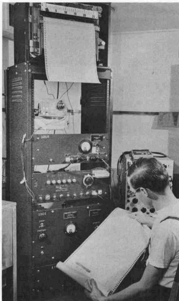
Figure 5. X-ray spectrum of polonium being recorded from proportional counter pulse height analyzer.
