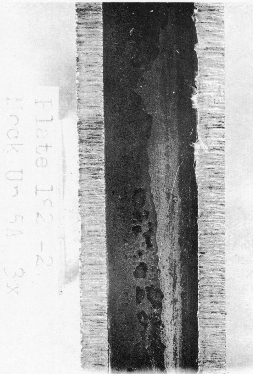
Fig. 54 Feed Stream Pipe Pitted Area 11 ft from Outlet (Hot) End (3X)
