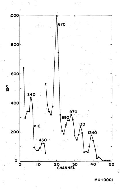
Fig. 12a. Gamma spectrum of Em<sup>211</sup>.
