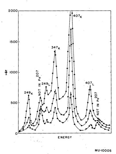
Fig. 9a. Radioactive decay of the conversion electrons of Po<sup>207</sup>.
