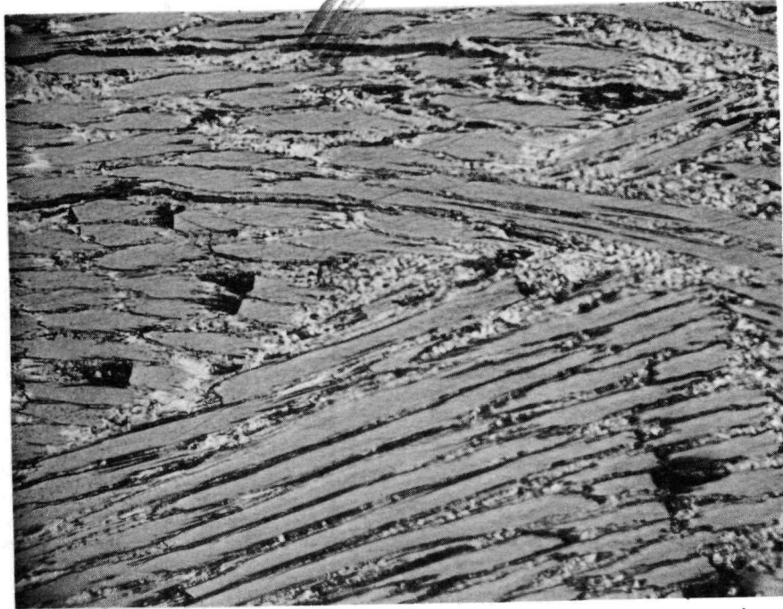
(a) Horizontal cross section view. No separation between graphite fibers or groups of differently oriented graphite fibers
