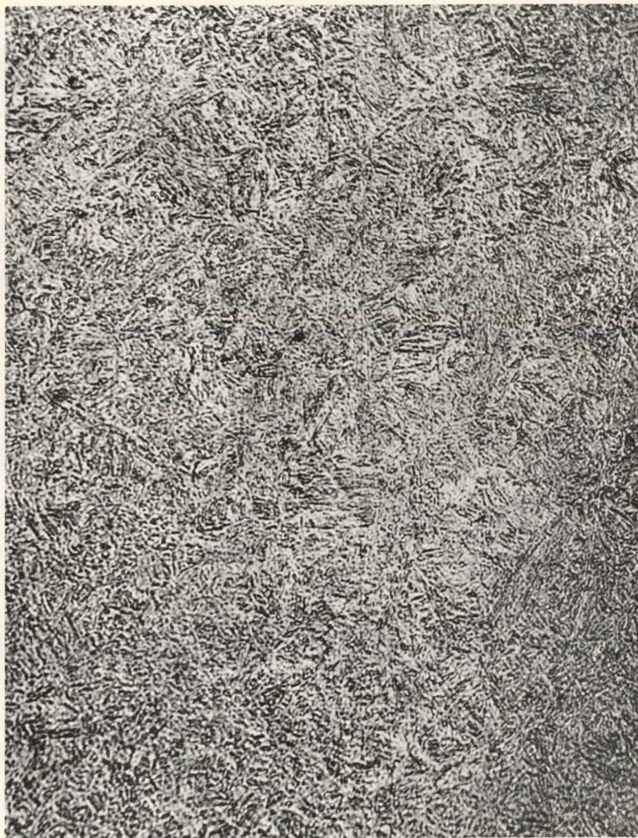
Fig. 16. Tempered Martensite Microstructure of 4340 (Etch 2% Nital, 1000X)
