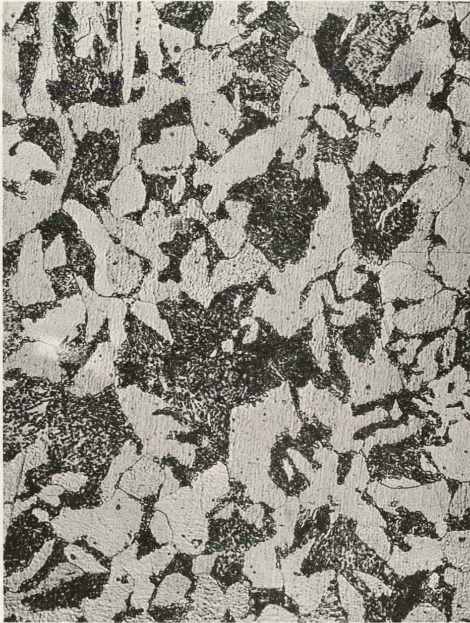
Fig. 24. Photomicrograph of 212-B Typical Ferrite and Pearlite Microstructure (Etch 2% Nital, 1000X)
