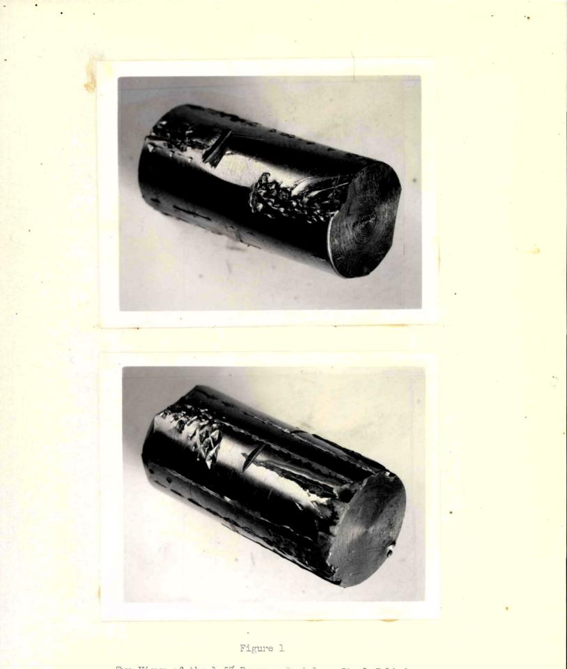
Two Views of the 1.5% Boron - Stainless Steel Cylinder Cooled in Liquid N<sub>2</sub> and Subjected to Impact with a Hammer and Chisel.
