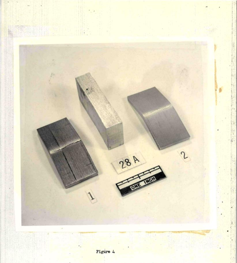
Photograph of Flexure Test Specimens and Coupon of 1.5% Boron - Stainless Steel From Which They Were Taken
