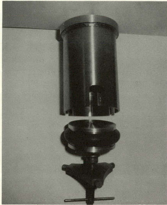
Figure 12. Leak testing fixture with seal mounted on plug.
