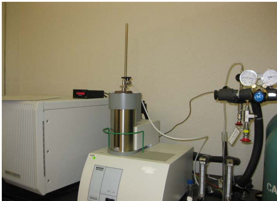
Figure 12- Experimental setup for measurements of noble gas adsorption
