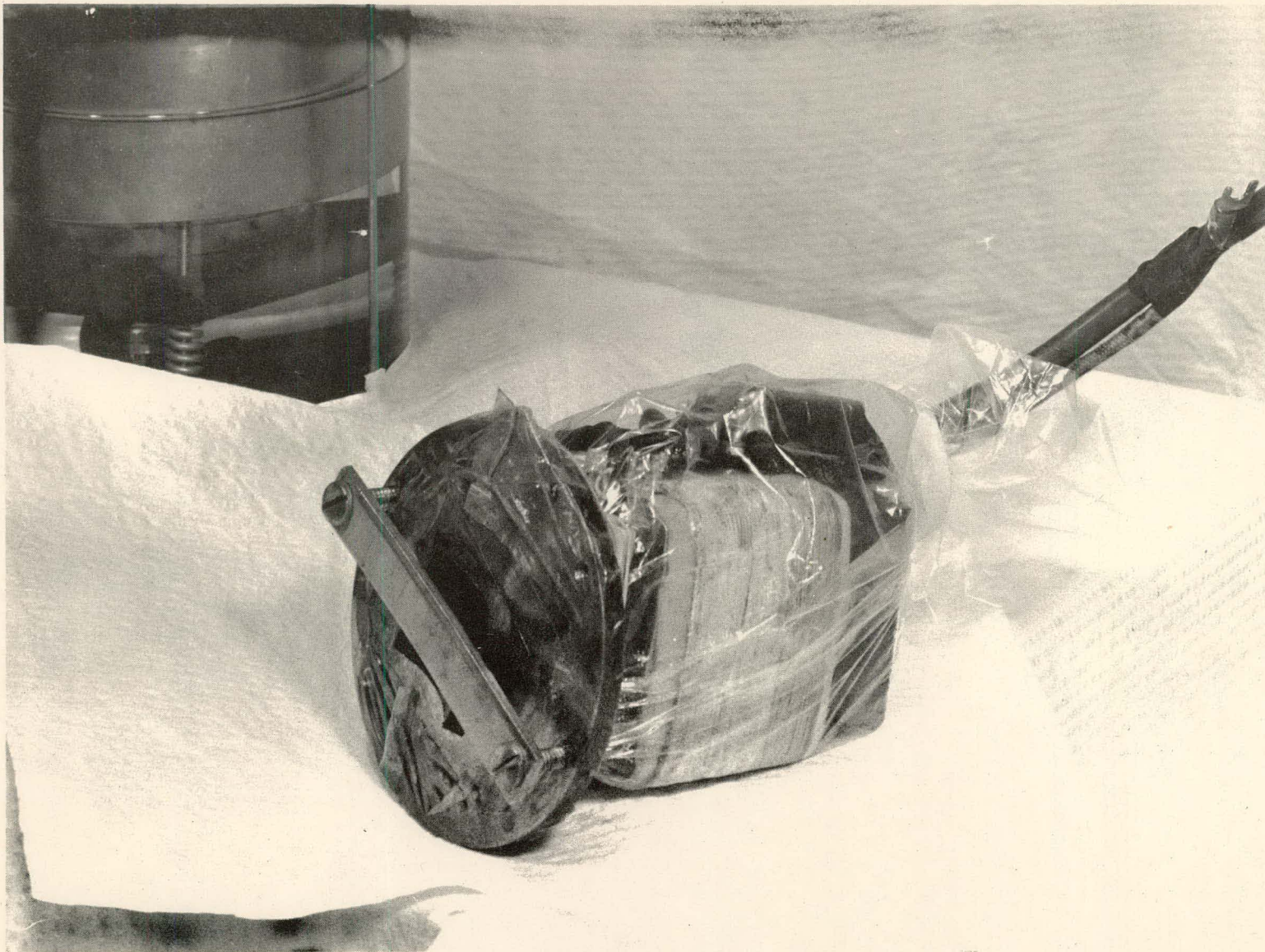
SPECIMEN CLAMPED TO MAGNETOSTRIKTOR
