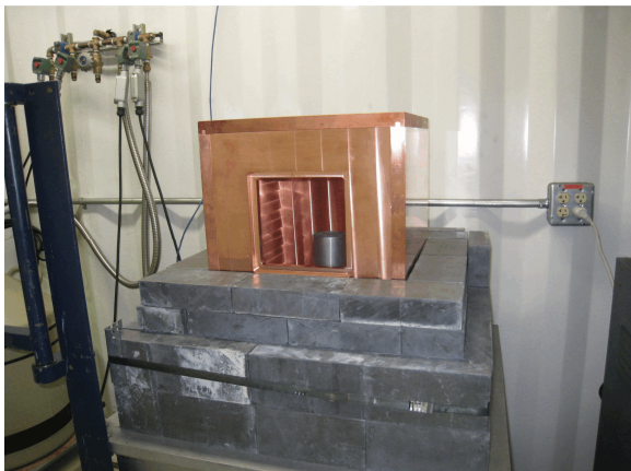
Figure 4: Inner copper shield of the Melissa detector
