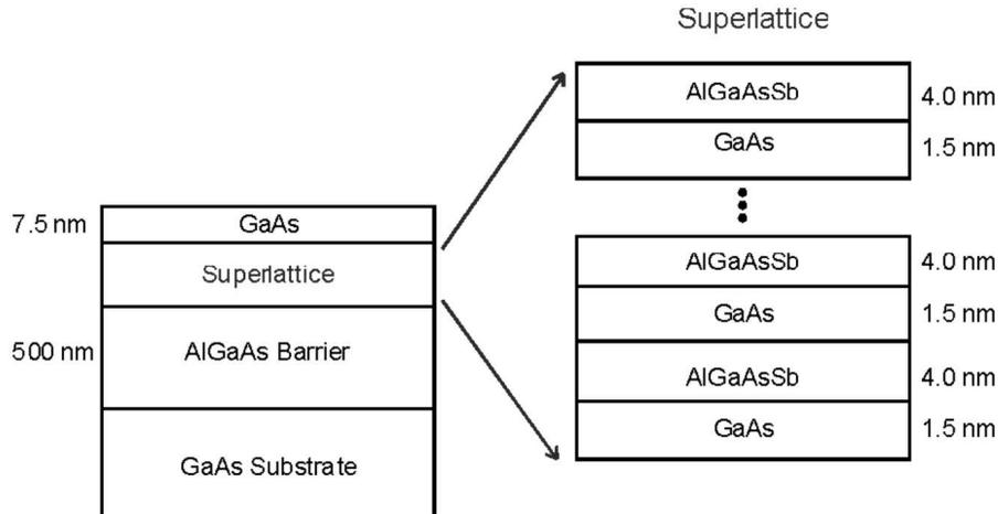
**FIGURE 1.** Diagram of the basic photocathode structure studied utilizing a superlattice consisting of GaAs wells and AlGaAsSb barriers.
