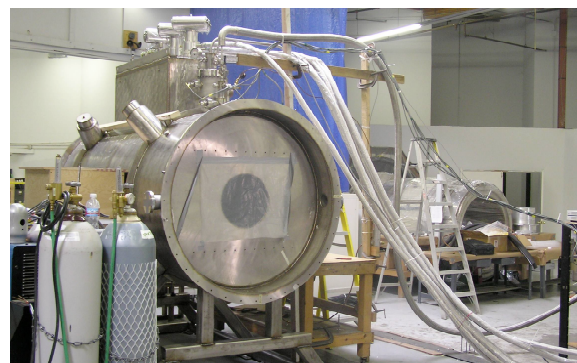
Fig. 2. Spectrometer Solenoid 1 with its Three PT-415 Coolers in Operation
