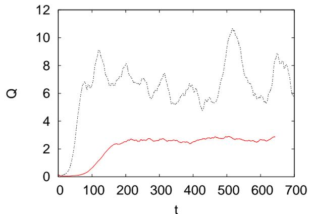
FIG. 4: (Color online) Comparison of line-averaged heat flux  $Q_{gk}$  versus time for QA\_35q (red solid) and NCSX (black dashed) from nonlinear GENE runs. QA\_35q achieves a reduction in turbulent transport over that in NCSX by a factor of about 2.5.
