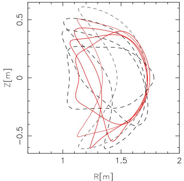
FIG. 3: (Color online) Comparison of boundary shapes of QA\_35q (red solid) and NCSX (black dashed) at values of  $N\zeta$  ( $=$  number of field periods  $\times$  toroidal angle)  $= 0, \pm\pi/2, \pi$ .
