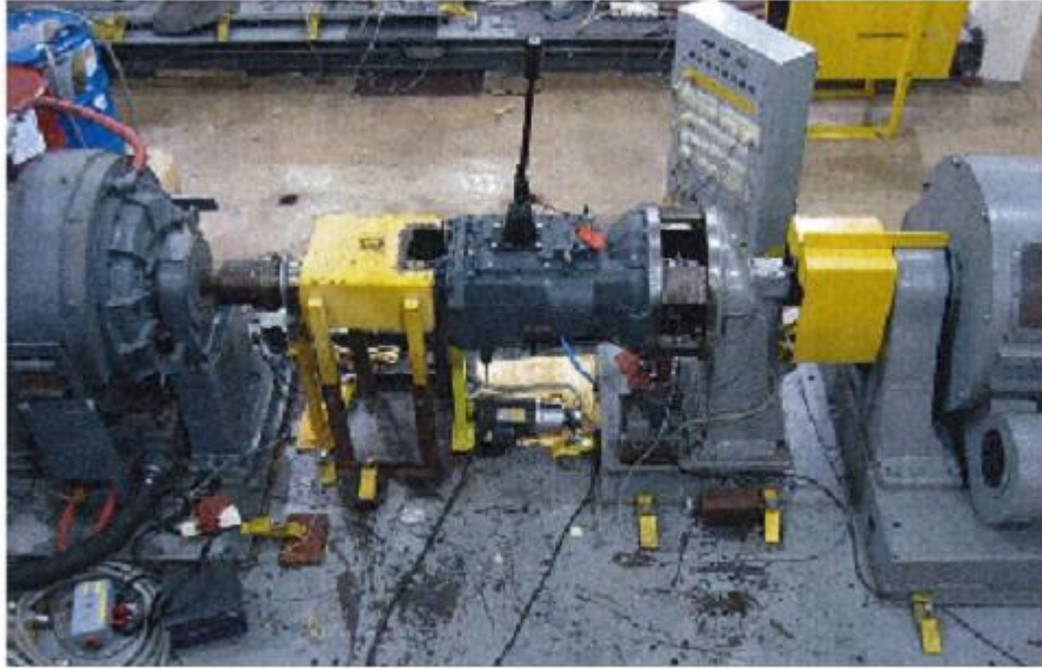
Figure 6.4.6-3: A standard Eaton transmission is mounted on the transmission efficiency dynamometer test stand at Southwest Research Institute.
