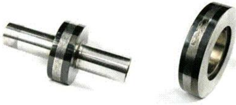
Figure 6.3.1-1: Because of improper machining, the PVD coating on these rollers was stripped off in 48 hours.
