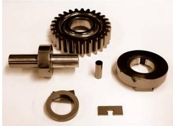
Figure 6.2.7-1: Eaton spur gear, contact fatigue rollers and Falex ring that have been coated with Diamond-Like Carbon by physical vapor deposition.
