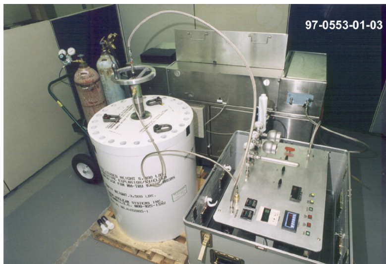
Figure G5-3. Headspace gas sampling of heated drum using Fourier transform infrared.
