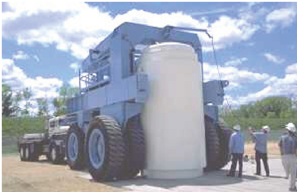
Figure E2-7. Dry storage cask transporter.
