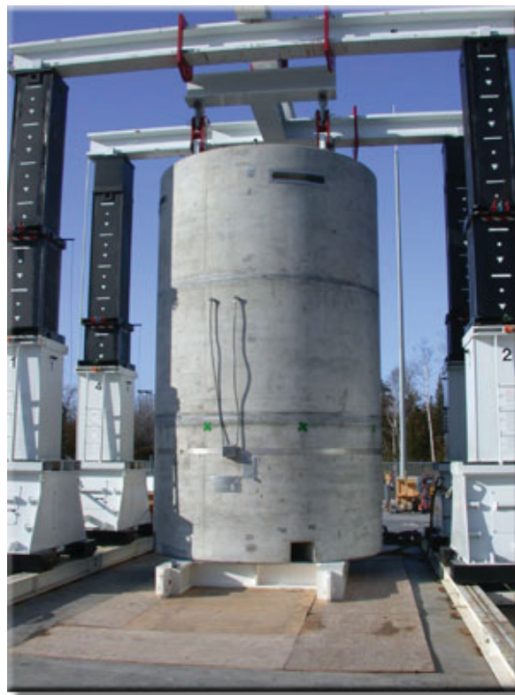
Figure G2-5. BNG Fuel Solutions vertical cask lift. Figure taken from BNG Web site.
