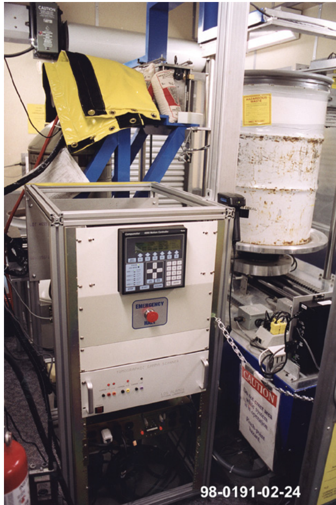
Figure G5-2. X-ray tomographic equipment for imaging drummed waste without opening the drum.
