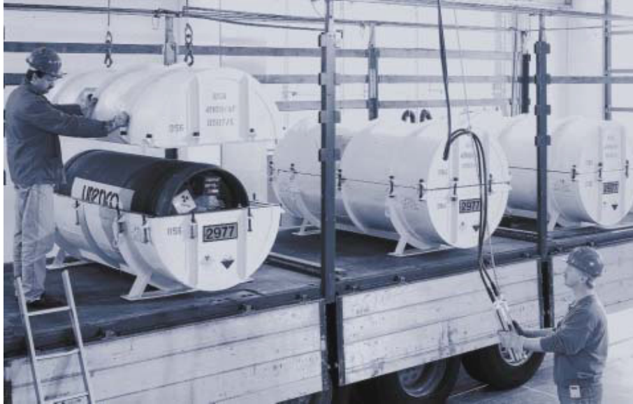
Figure C1-11. Enriched UF_6 product container being loaded into an overpack for shipment.
