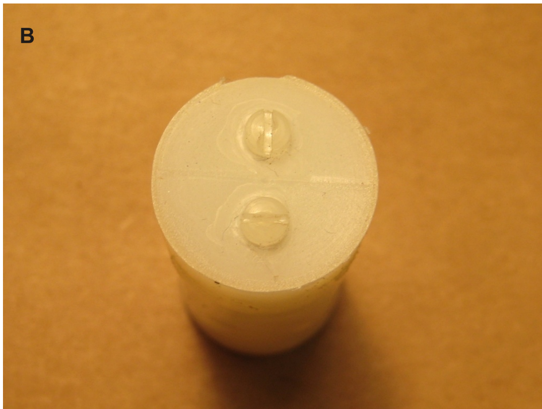
Fig. 6.12: (A) Diagram of sealed nylon phantom. Dashed lines outlining the pattern indicate that the material is opaque. Shaded area in figure is the pattern machined into the two halves, which are joined along the dotted line. (B) Photograph of one such phantom. Sealing line is visible horizontally between the screws.
