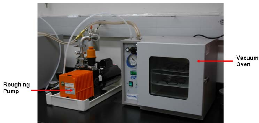
Figure 6: Temperature controlled oven with vacuum supplied by roughing pump
