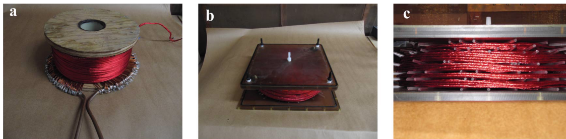
Figure 3.1: Images of early polarizing coil designs. a. Image of a late model open bore polarizing coil. Note peripheral cooling with copper wires and use of litz wire. b-c. Bottom and side views of late model LN 2 cooled coil. Coolant flows into the center, through a manifold into the channels (shown in c ) which are held open with soft plastic sticks during winding. Each turn of wire has a cooling channel on one side to avoid formation of hot spots.
