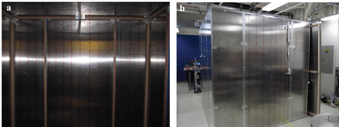
Figure 3.6: Images of 1.6 mm aluminum shield. a. Photograph of interior of 1.6 mm aluminum shield, showing wooden supports. b. Photograph of exterior of 1.6 mm aluminum shield. The 4 vertical walls are designed to be symmetrical to avoid disorting the shield response to the prepolarizing pulse.
