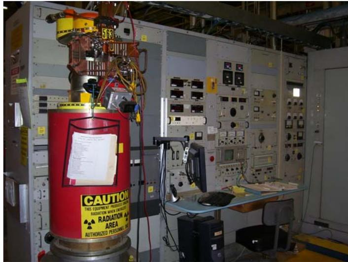
*Figure 1: A test station with a klystron.*
