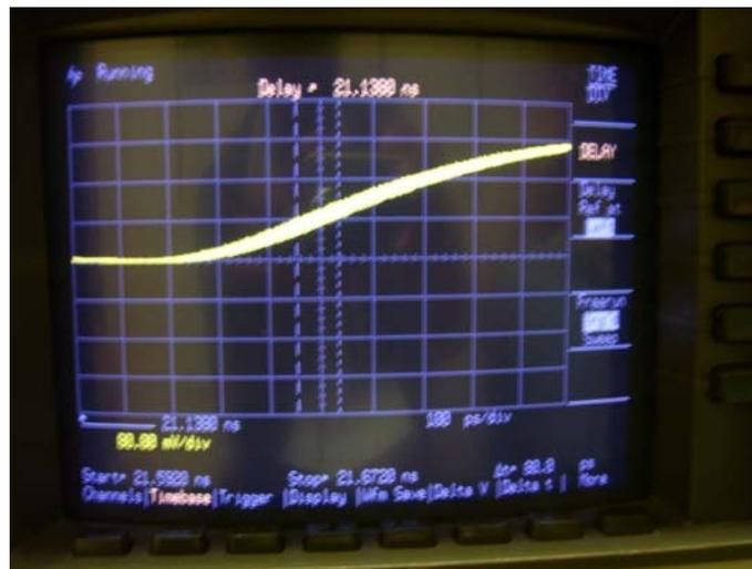
Figure 4: Non-DCM Channel jitter measurement.
