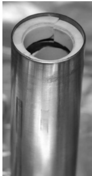
Figure 5. Dummy cell after vibration testing
