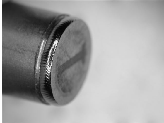
Figure 7. Welded tungsten tube joint
