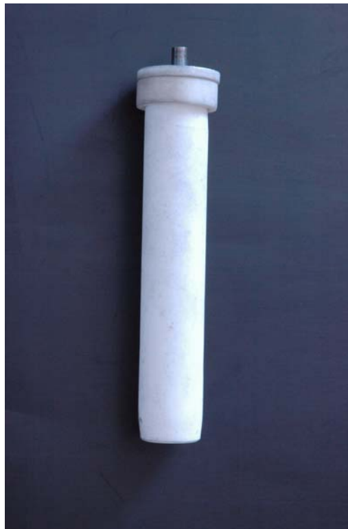
Figure 9. Cathodic compartment; beta \alpha - alumina tube glass bonded to alumina header and alumina header bonded to alumina top.
