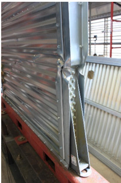
(c) Chord framing member buckles
