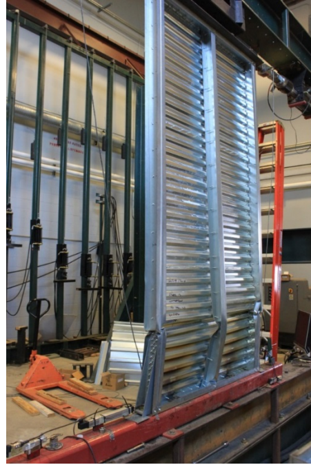
(b) Vertical Framing member buckle
