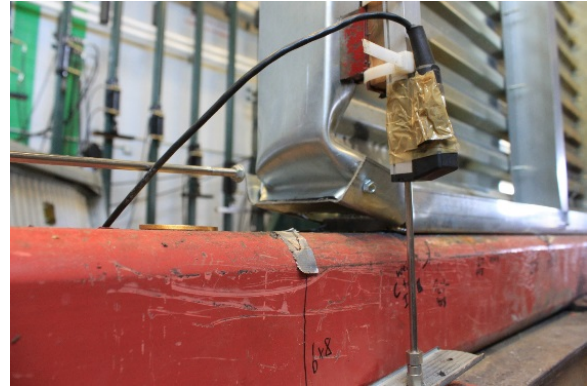
(b) Chord framing member lift up
