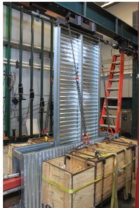
(a) Wall specimen without gravity load (b) Wall specimen with gravity load Figure 4.3 - Back View of Test Setup
