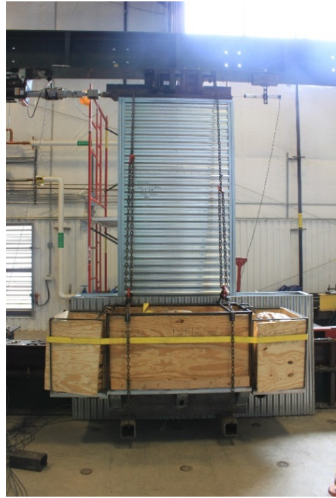
(a) Wall specimen without gravity load (b) Wall specimen with gravity load Figure 4.2 - Front View of Test Setup
