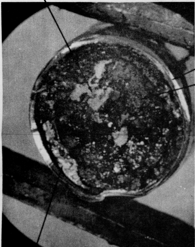
TRANSVERSE SECTION PORTION OF NICKEL RING
