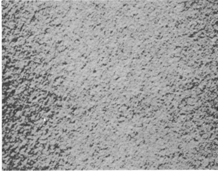
FIGURE 4.6 SURFACE SCALE FORMED ON 20% COLD WORKED, TYPE 304 STAINLESS STEEL SPECIMEN, X 15
