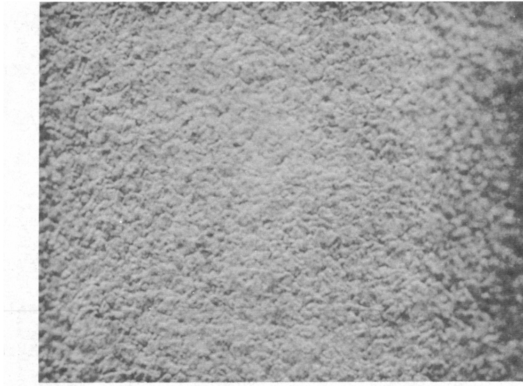
FIGURE 4.2 SURFACE SCALE FORMED ON ANNEALED TYPE 304 STAINLESS STEEL SPECIMEN, X 15
