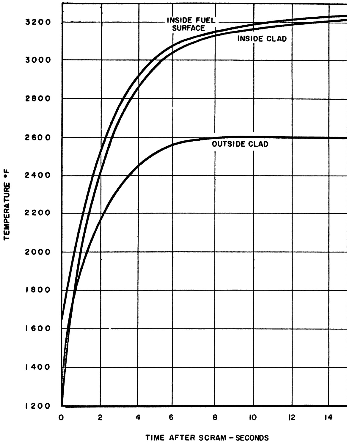
CLAD & FUEL SURFACE TEMPERATURE VS. TIME AFTER SCRAM FOR ZERO FLOW
