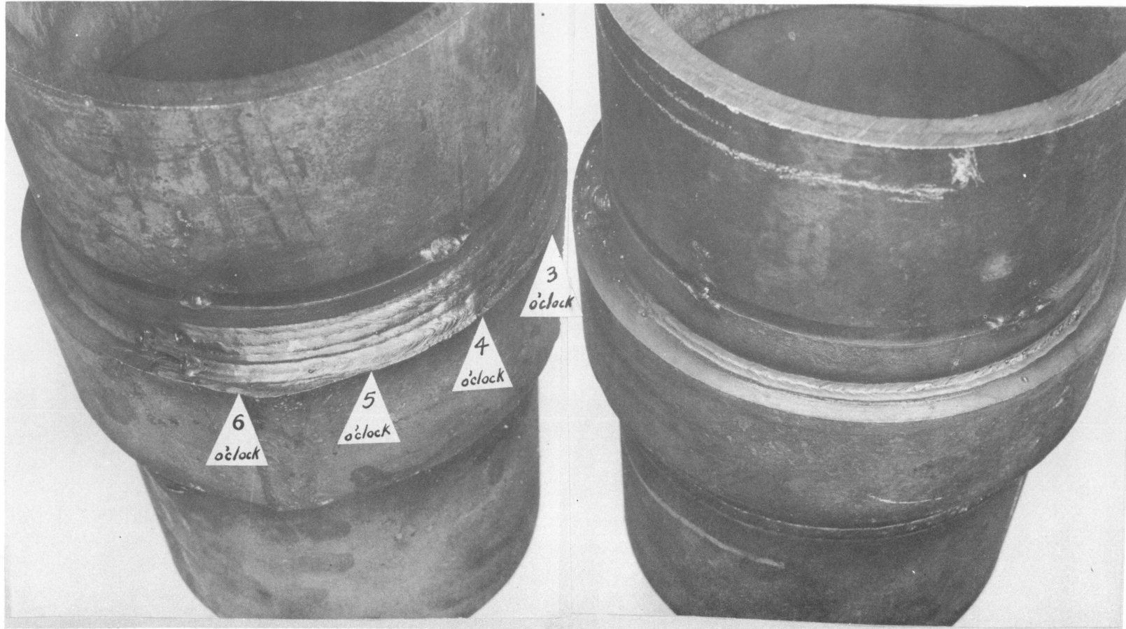
FIG. 57: GAS-SHIELDED METALLIC ARC WELD IN CROLOY 2-1/4 PIPE 6-1/2 in. OD x 3/8 in. WALL
