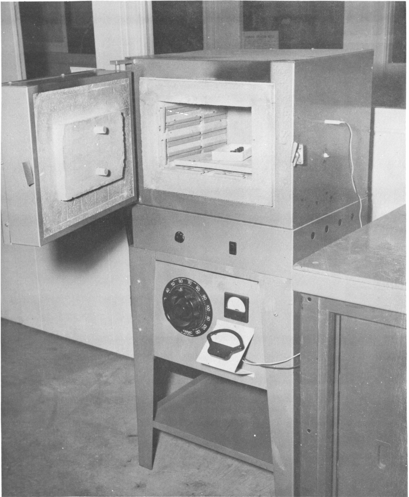
FIG. 48: ELECTRIC FURNACE AIR ATMOSPHERE
