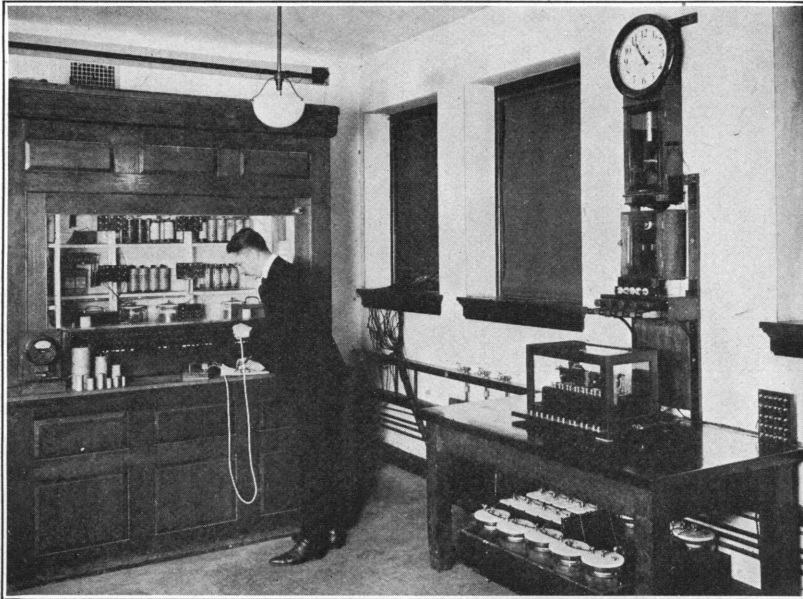
FIG. 63.— Automatic life tests of dry batteries
