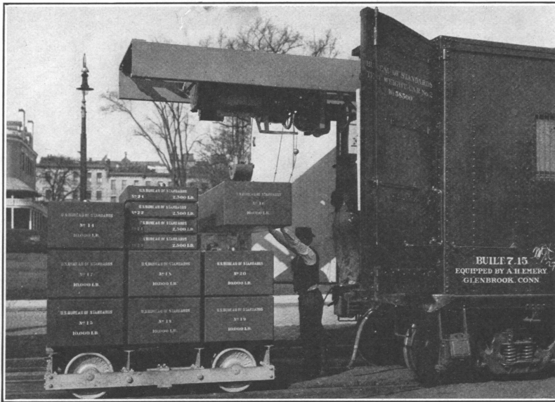
FIG. 24.—Track scale test car equipment
