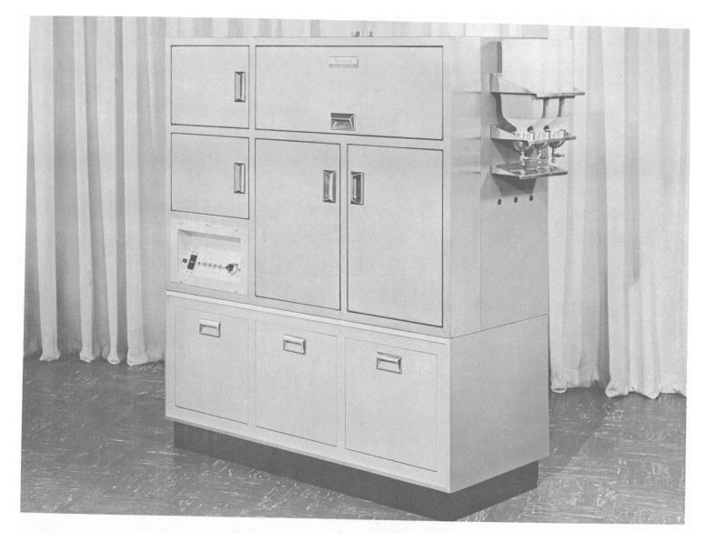
Figure 18. Minicard Film Processor
