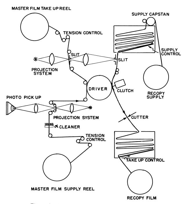
Figure 5. Rapid Selector Film Transport Schematic
