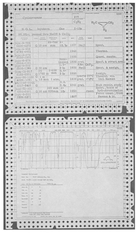
Figure 3. Spectral Data Card
