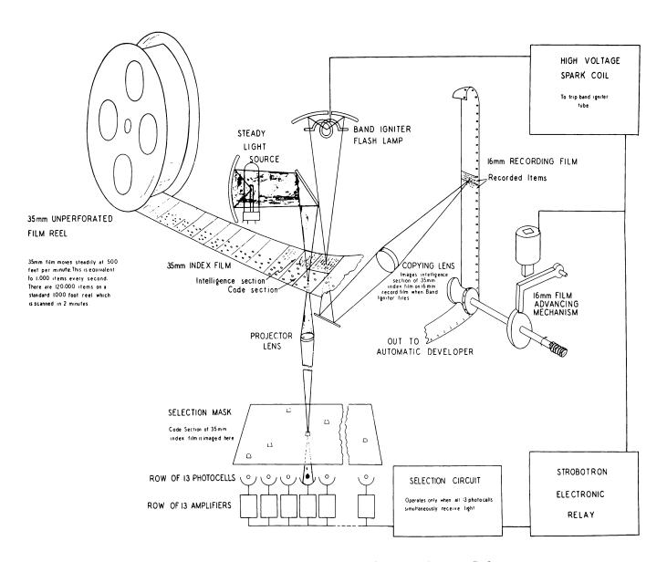
Figure 1. Schematic Diagram of Bush Rapid Selector
