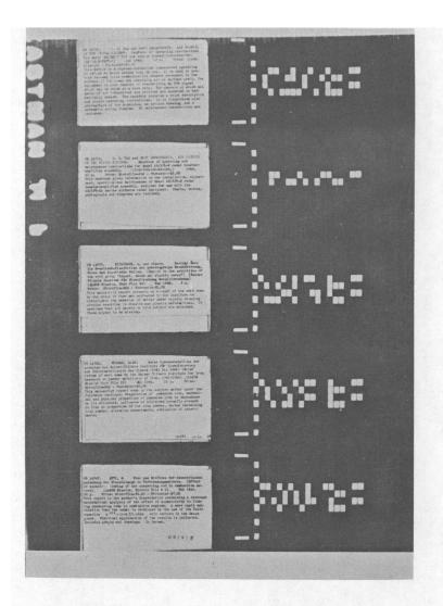
Enlargement of Microfilm Showing Format Used by ERA's Rapid Selector Design
