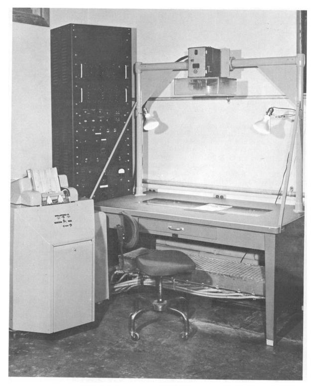
Figure 4. Rapid Selector Encoder
