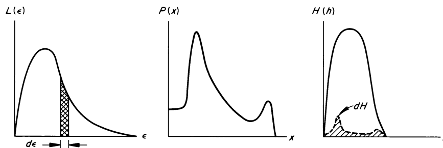
Fig. 14.5. Contribution of dH from Each Interval d\epsilon of LET Spectrum Has the Shape of the Track-Length Distribution P(x) .
