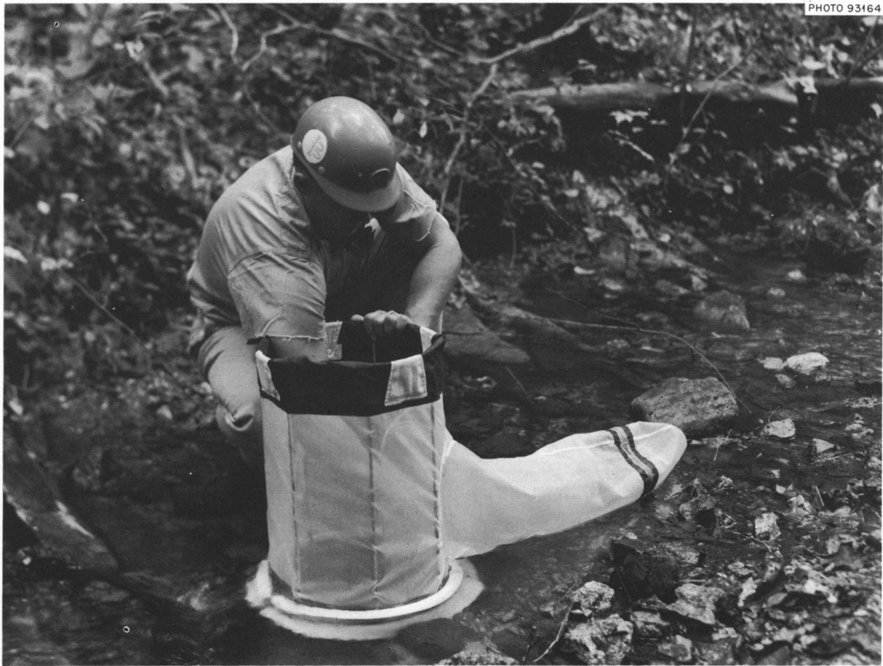
Fig. 12.14. Bottom Sampler Used in Sampling Benthic Macroinvertebrates in Walker Branch Watershed Streams. Sampling area of the cylinder is 0.10 \text{ m}^2 .
