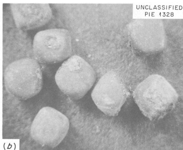
Fig. 13.3. Original Arc-Fused Pellets and Those Irradiated Under \text{D}_2\text{O} . Exposure: 2.5 \times 10^{18} fissions/gram. (a) Original; (b) irradiated. 3.3X. Reduced 15%.
