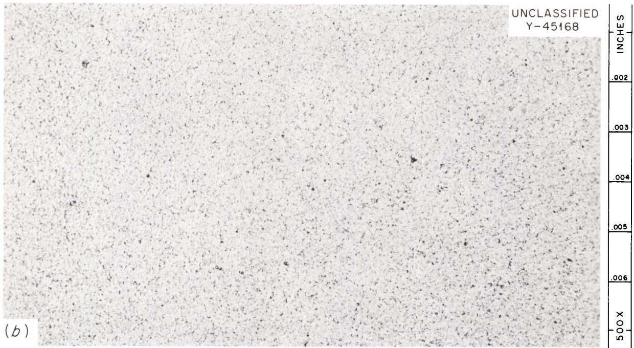
Fig. 6.2. Sol-Gel E: \text{ThO}_2 -4.5 wt % \text{UO}_2 Powder. No impurities were found in this material. Small surface cracks may be seen in the particles. (a) 150X. As polished. (b) 500X. Etchant: boiling \text{HNO}_3 -HF. At higher magnification the particles show a very fine natural porosity and extremely fine crystallites (spheroidal white particles). No large grain boundaries are evident.
