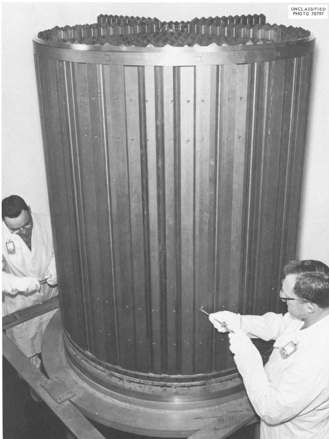
Fig. 1.1. Assembly of the MSRE Graphite Core.
