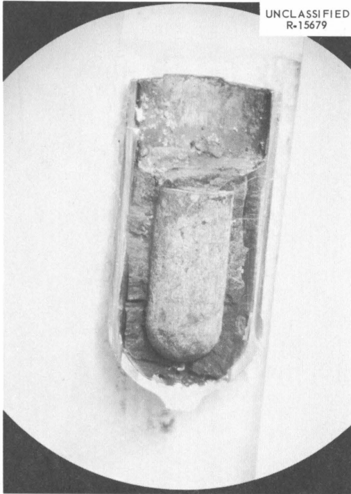
Fig. 5.14. Capsule 4, Showing Graphite Bearing Shiny Film.
