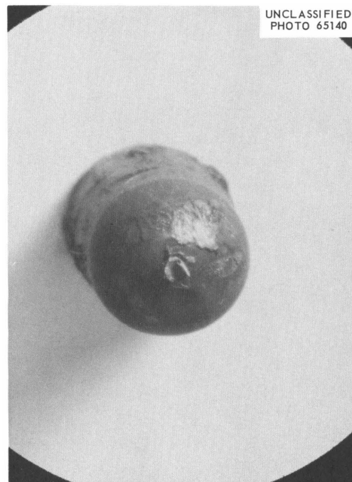
Fig. 5.13. Scale on Bottom of Graphite Core from Capsule 3. Projection from Center is Part of the Metal Supporting Pin.
