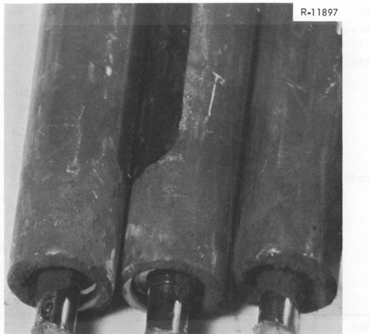
Fig. 3.13. Lower End of Experiment 5 Specimens Following Irradiation; After Disassembly.
