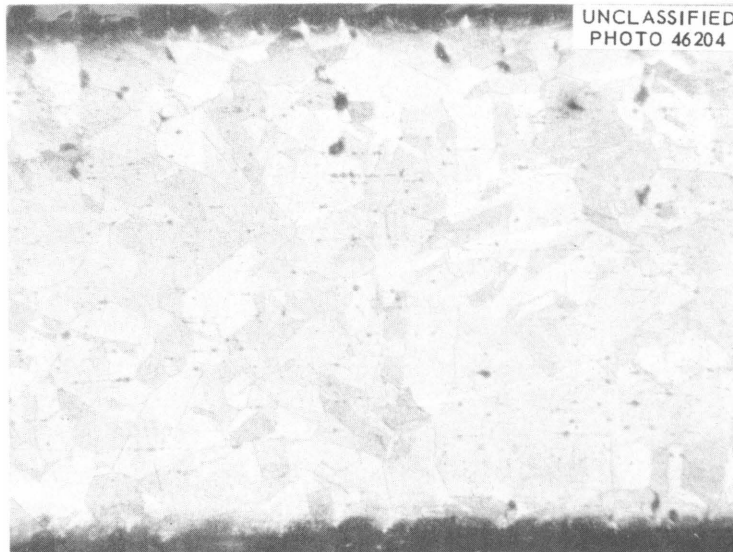
Figure 21 (9) . Cross-Section of Chromel P Wire Taken from Ceramic Beaded Assembly in One Foot, 0.250-in.-O.D. Inconel Protection Tube After 5000 hr at 1800°F. UT Sample No. 123. Etchant: \text{CuCl}_2 - aqua regia solution. 100X
