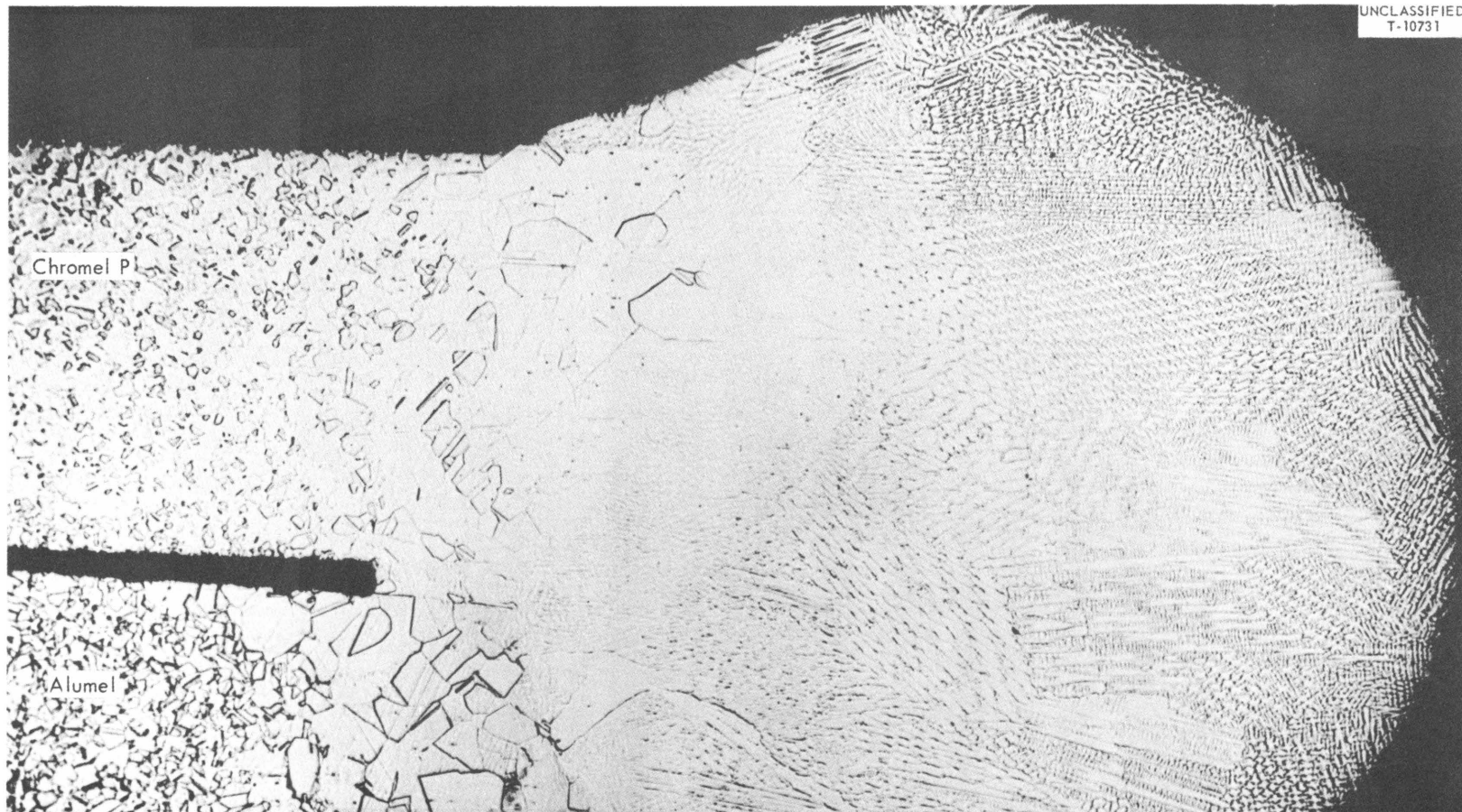
Figure 27. Cross-Section of Chromel P-Alumel Thermocouple Junction Where Wires Were Carefully Cleaned of Any Oxide Prior to Junction Formation. (Note absence of any deposits in Chromel P Wire.) Reduced 21%.
