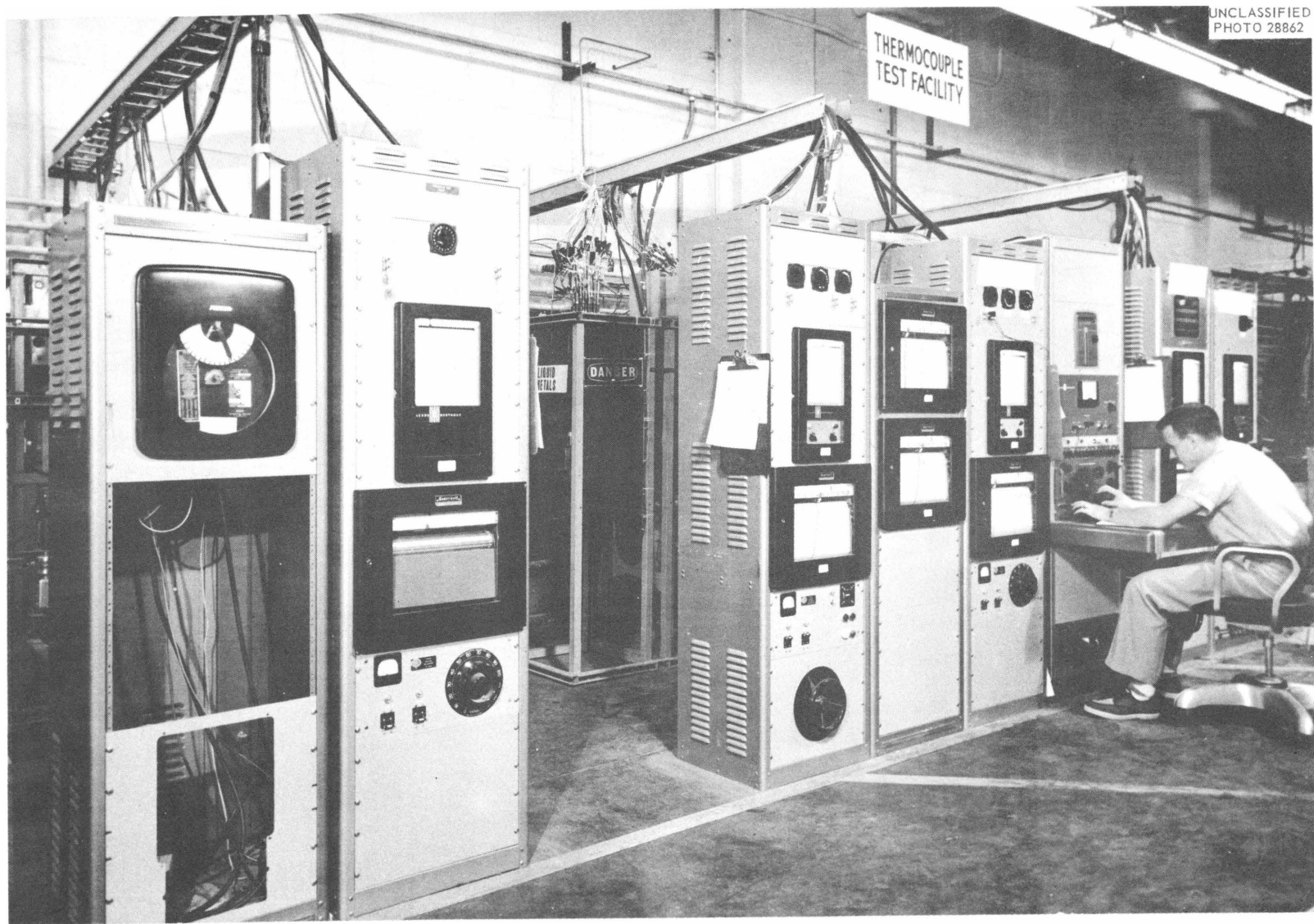
Figure 5. Facility for NaK, Na, Fluoride Salt Aging and Calibration of 0.250-in.-O.D. Sheathed and Well-Type Thermocouples. (Uncompleted cabinet will contain the controls for a eutectic salt melting point apparatus.)
