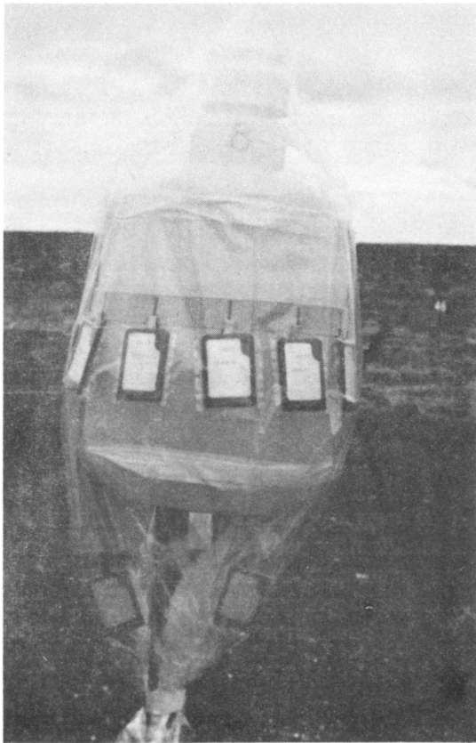
Fig. 13 Phantoms approximating man's torso in size and composition.
