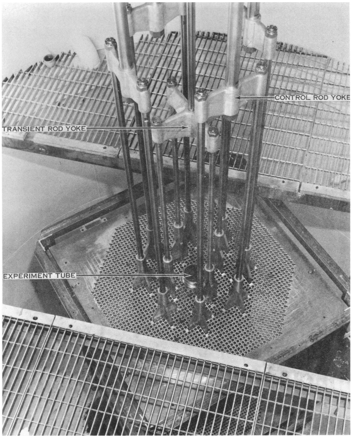
Fig. 4 CDC support structure assembled in the Spert I reactor vessel. View showing control and transient rod yokes.
