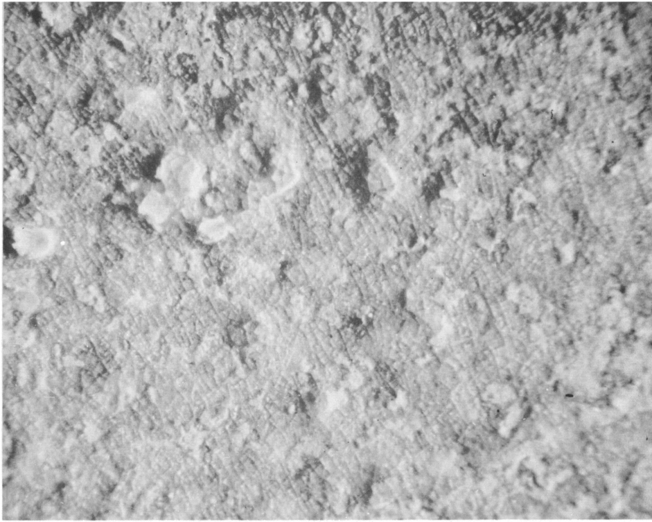
Fig. 12 Aluminum oxide film after irradiation. Although spalling took place, the coatings increased in thickness. A boehmite structure was detected.
