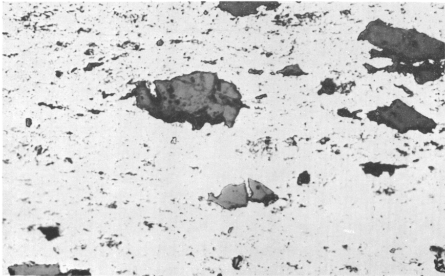
AS POLISHED BEFORE IRRADIATION 500X
