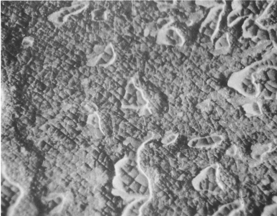
Fig. 13 Aluminum oxide film after irradiation exhibiting spalled and nonspalled areas.
