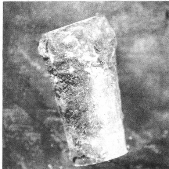
Figure III-15 Corroded spacer after sectioning magnification - 4 x
