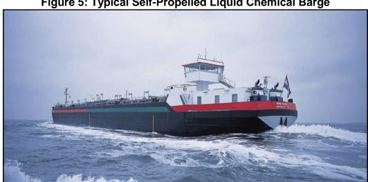
Figure 5: Typical Self-Propelled Liquid Chemical Barge
