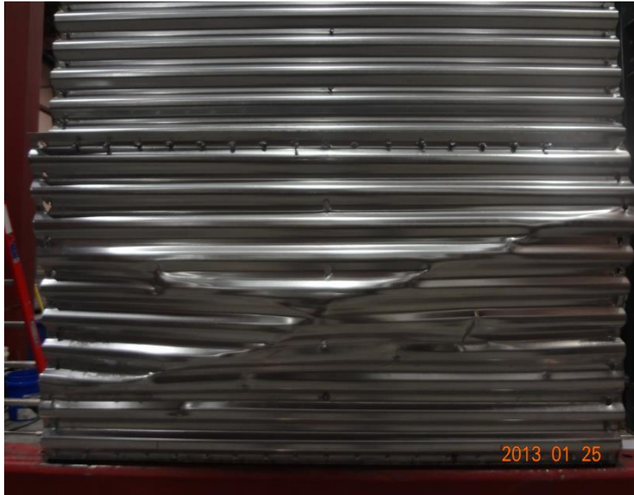
Figure 26. Failure mode of wall configuration Type 1
