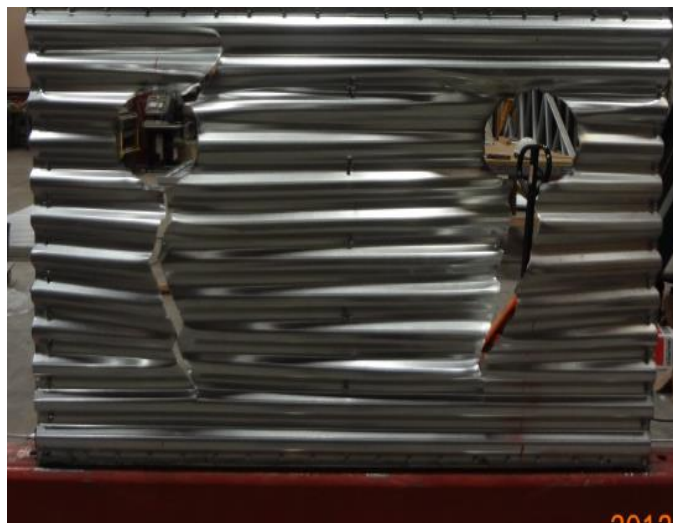
Figure 29. Failure mode of wall configuration Type 3
