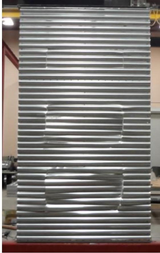
Figure 31. Failure mode of wall configuration Type 5
