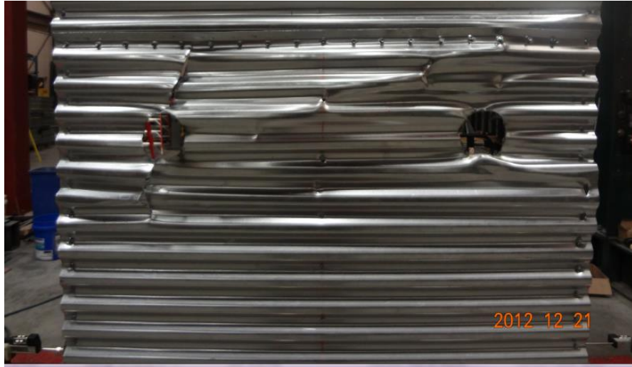
Figure 30. Failure mode of wall configuration Type 4
