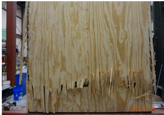
Figure 39. Failure mode of plywood wall of configuration Type 12
