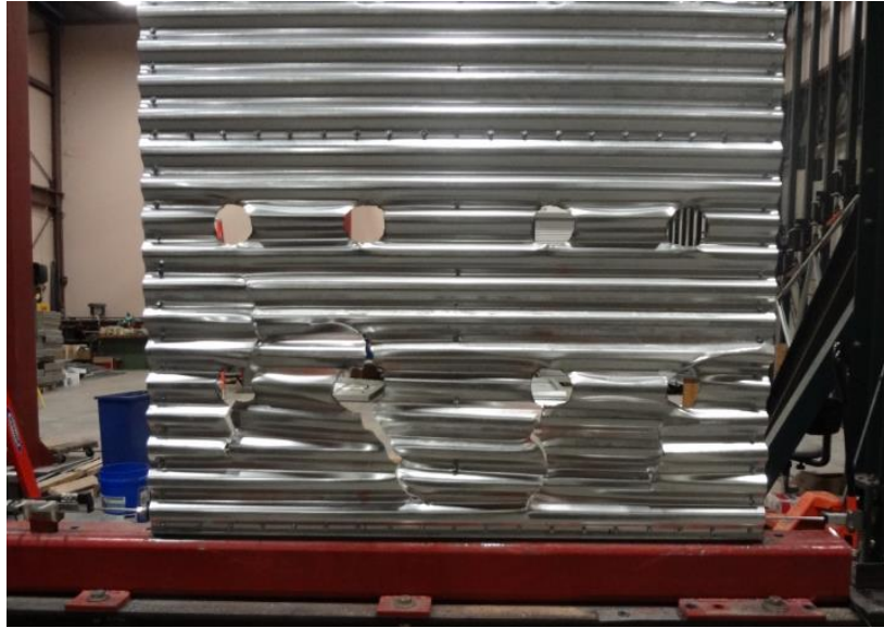
Figure 32. Failure mode of wall configuration Type 6
