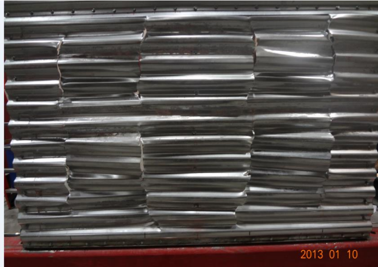
Figure 33. Failure mode of wall configuration Type 7
