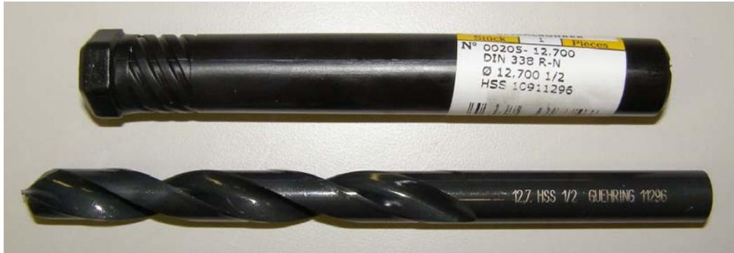
Figure 2: High Speed Steel Drill Bit
