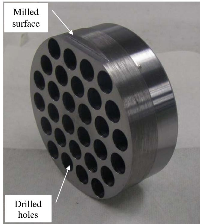
Figure 9: Drilled Workpiece
