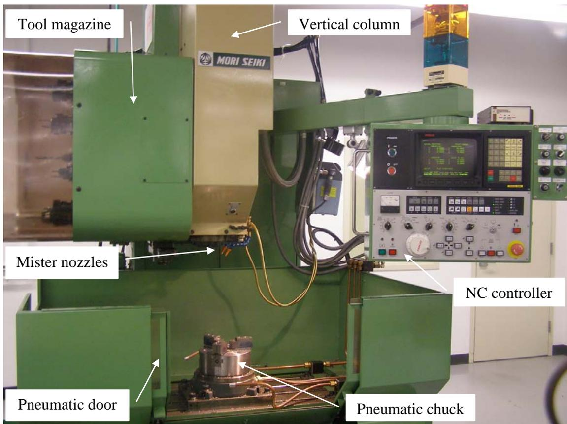
Figure 8: Mori Seiki Vertical Milling Machine
