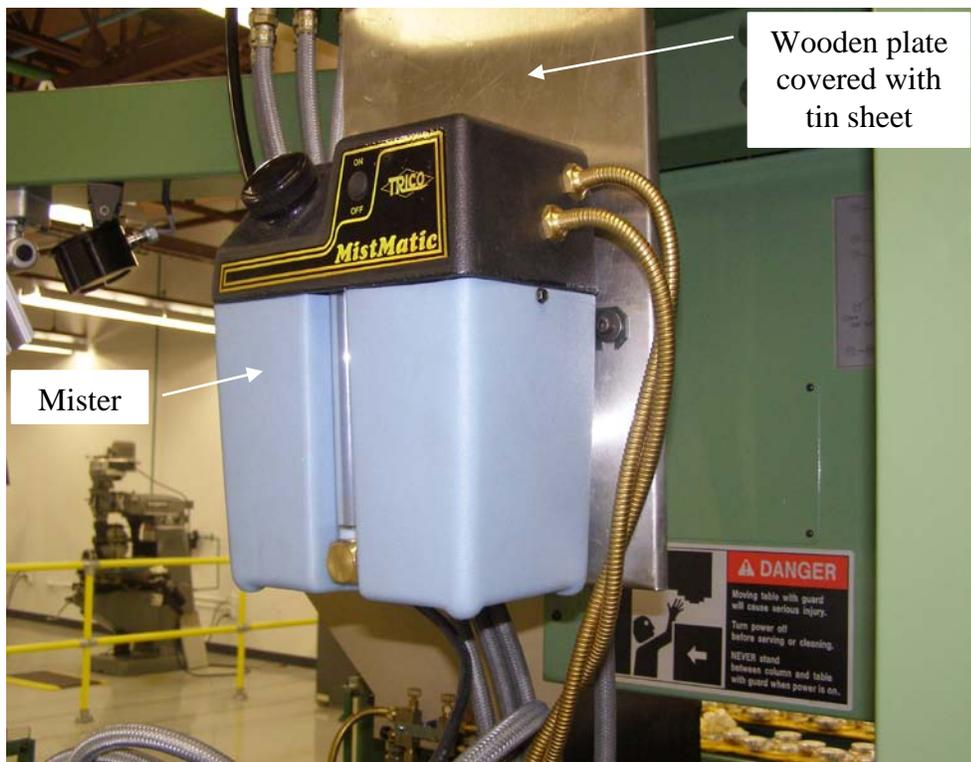
Figure 7: Mister Assembled on CNC Milling Machine
