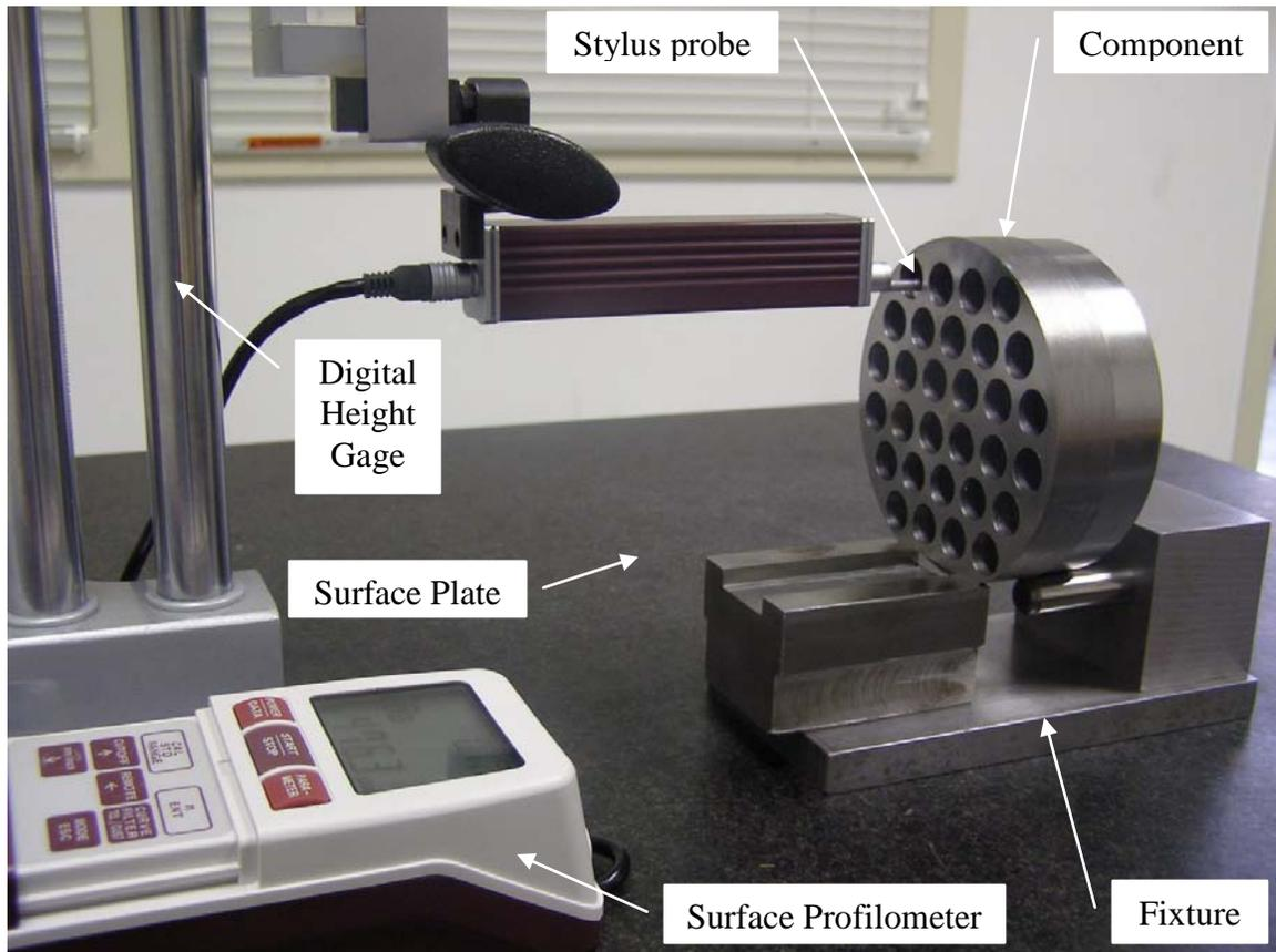
Figure 10: Measurement of Surface Roughness
