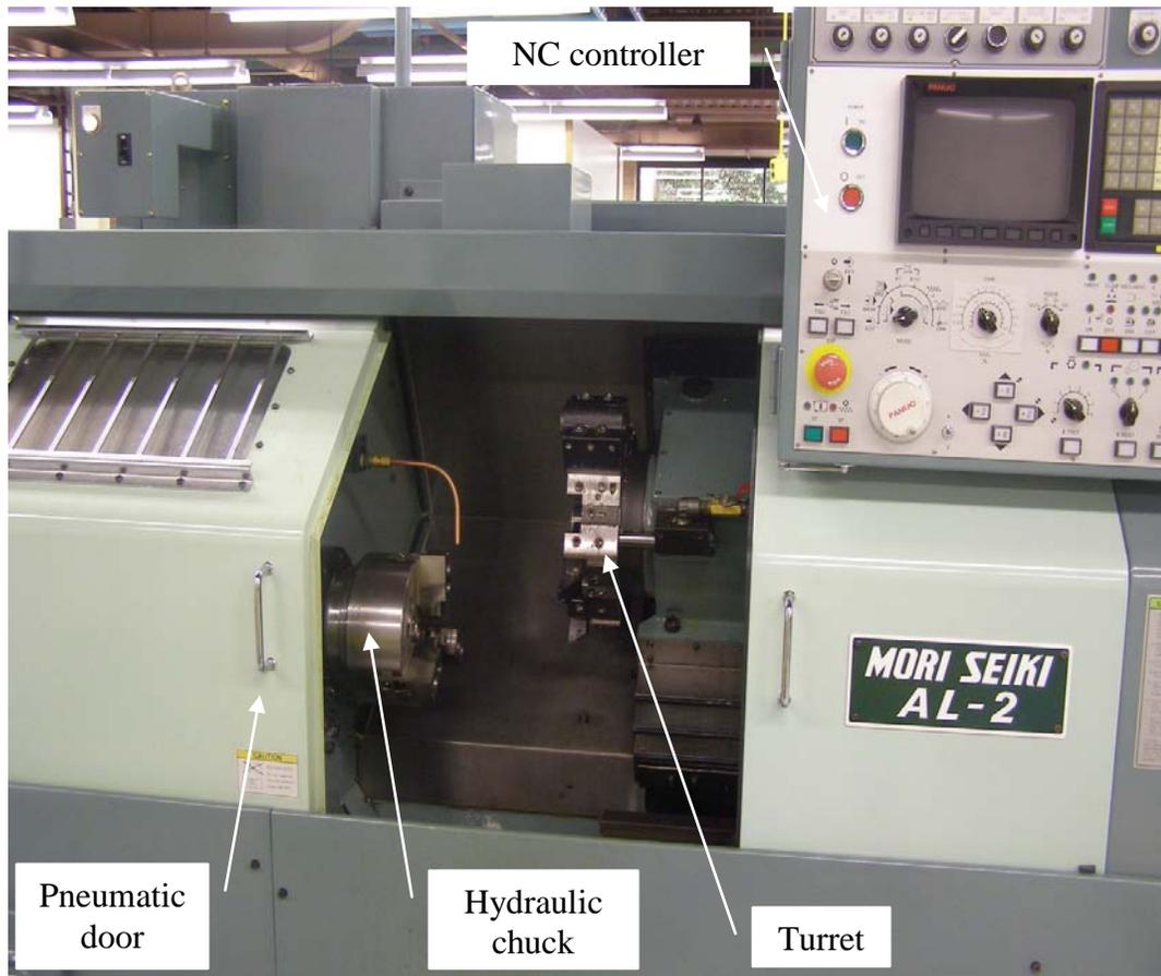
Figure 5: CNC Lathe
