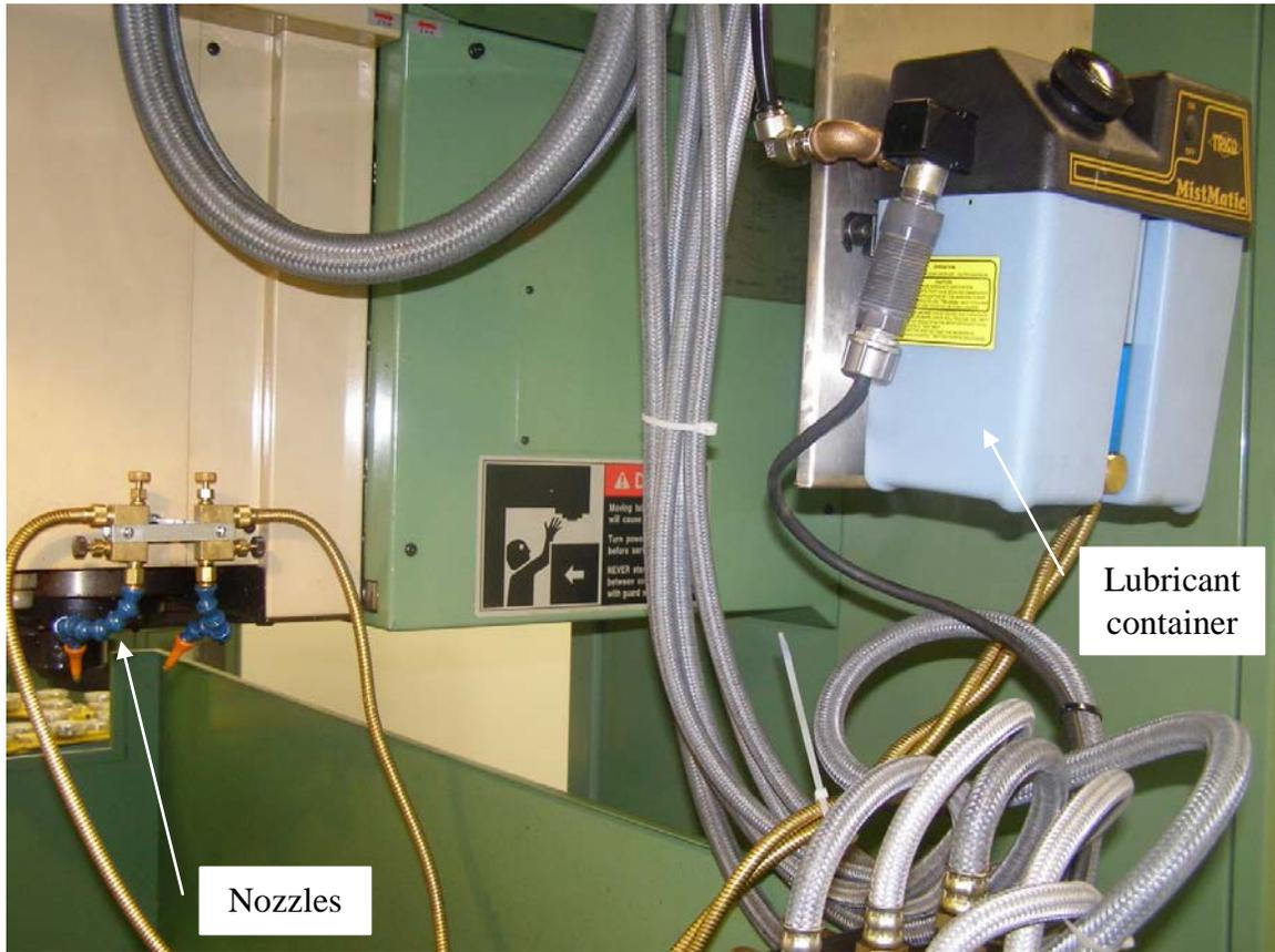
Figure 1: External Spray MQL System
