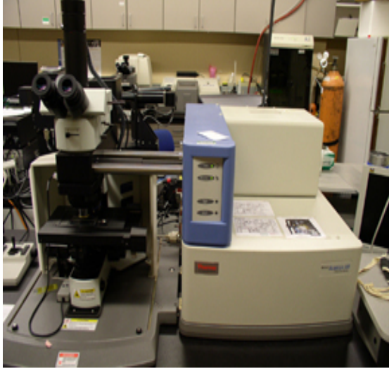
Figure 3-1. (a) Raman Spectrometer (UNT-CART) (b) Raman sample structure Raman spectroscopy is one of the most widely used techniques to understand the local
