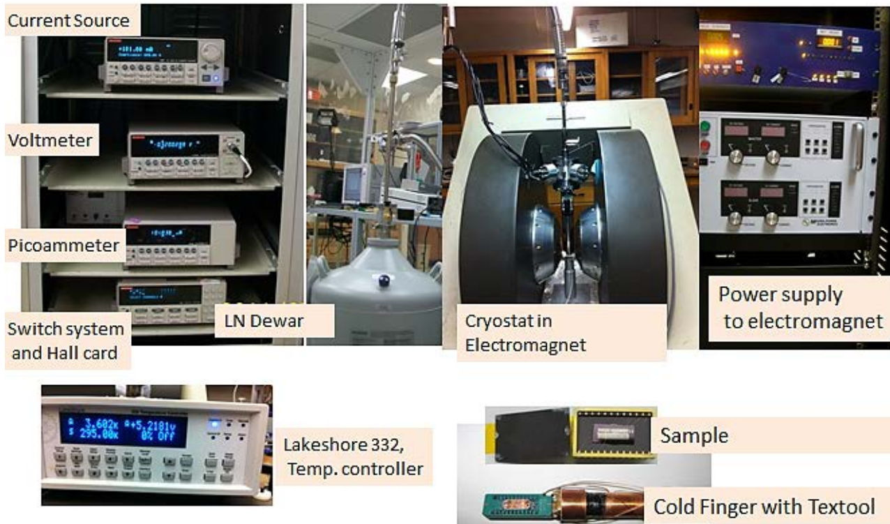
Figure 2-5. Resistivity and Hall Effect measurement Equipment (photograph). Resistivity can be also be determined by using the Van der Pauw technique 45,46 . This
