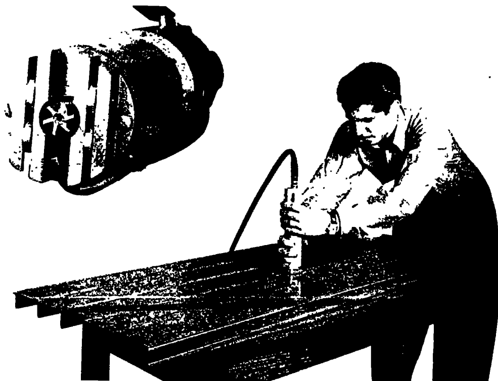
Figure 21.- End-milling tool for removing the protruding portion of the rivet head.
