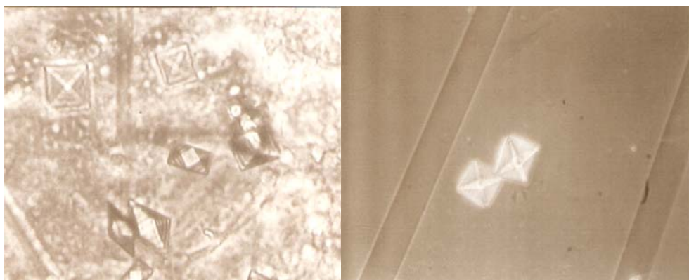
Figure 20. Large medium precipitates have a characteristic crystalline shape. 200x magnification.
