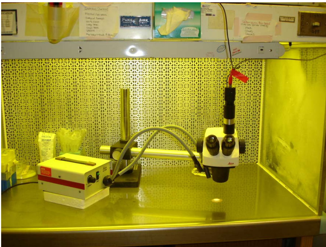
Figure 23. Open vent hood for microdissection of embryonic mouse brains. Separate hoods are necessary for mouse sacrifice, microdissection, and media preparation and culture handling in an effort to prevent cross-contamination.
