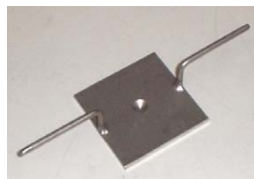
Figure 6. Stainless steel flaming mask with 2.5 mm diameter opening.
