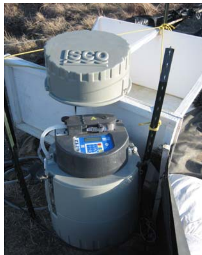
Figure 10. ISCO™ automated sampler with collection bottles stored in the bottom.
