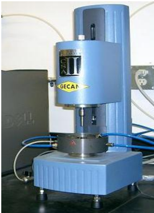
Figure 22: Image of dynamic shear rheometer Courtesy: Gecan, 2007
