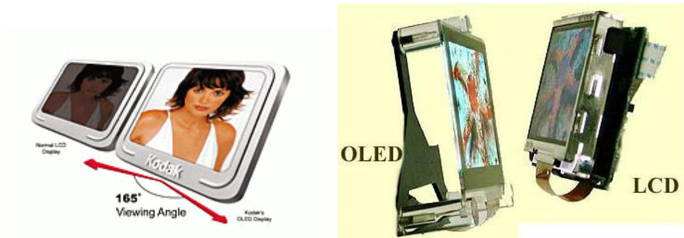
Figure 8: The brightness and view angle of LCD and OLED
