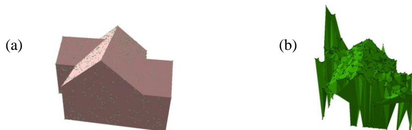
Figure 16. 3D B6 Models: (a) User-generated 3D model; (b) TIN model from LiDAR.
