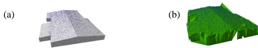
Figure 14. 3D B3 Models: (a) User-generated 3D model; (b) TIN model from LiDAR.
